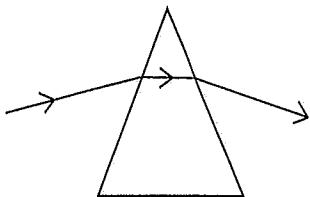
(So far we have ignored the fact that different wavelengths – different colours – of light travel at different speeds through media like glass. This causes different angles of refraction, leading to a spectrum being produced from white light.)
