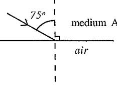
Answer: The sine of the angle of refraction works out to be greater than one. This is impossible. No refraction occurs.
