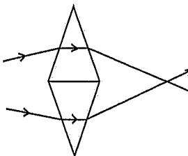
It is not a major step to see how curved, rather than straight, surfaces can focus all the rays from an object at one image point.
